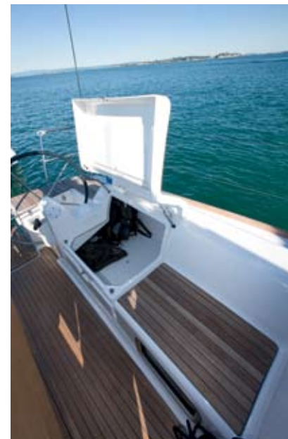
The port and starboard lockers offer good stowage and don't intrude into the aft cabins
