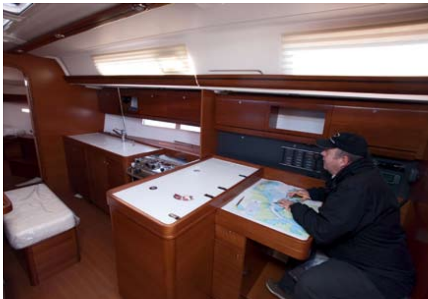
The nav station is the ideal spot for a laptop and there's plenty of space for additional electronics. The refrigeration is between the stove and the chart-table. Fridge access is via two top hatches or the front door on the for'ard end of the unit
