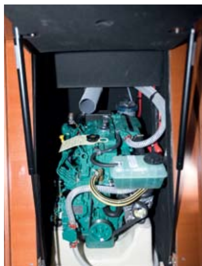
The engine compartment is well insulated with good access for routine maintenance
